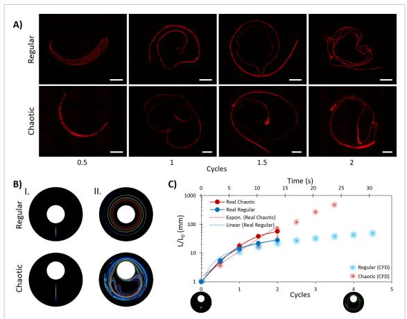
**Figure 2.** Chaotically printed fibers and CFD simulations. (A) Fluorescence micrographs of GelMA fibers fabricated through regular and chaotic arrangements and at different numbers of cycles in a miniJB device (270°, 810°). Scale bar: 2 mm. (B) CFD simulations of the deformation of centerlines caused by regular and chaotic flows (I) before and (II) after five cycles (270°, 810°) and (C) comparison between elongation of experimental fibers against CFD predictions.
